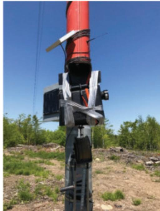
Picture 8 – AB8 Survey Station (installation)
