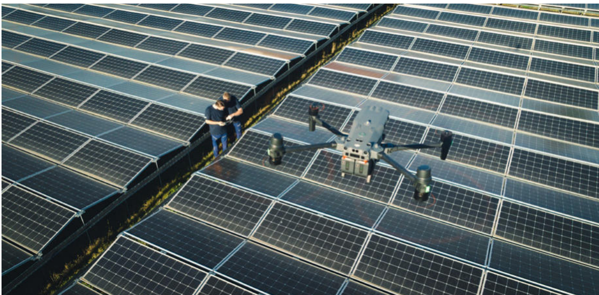
Engineers use a drone with a thermal imaging camera to search for defective modules.
