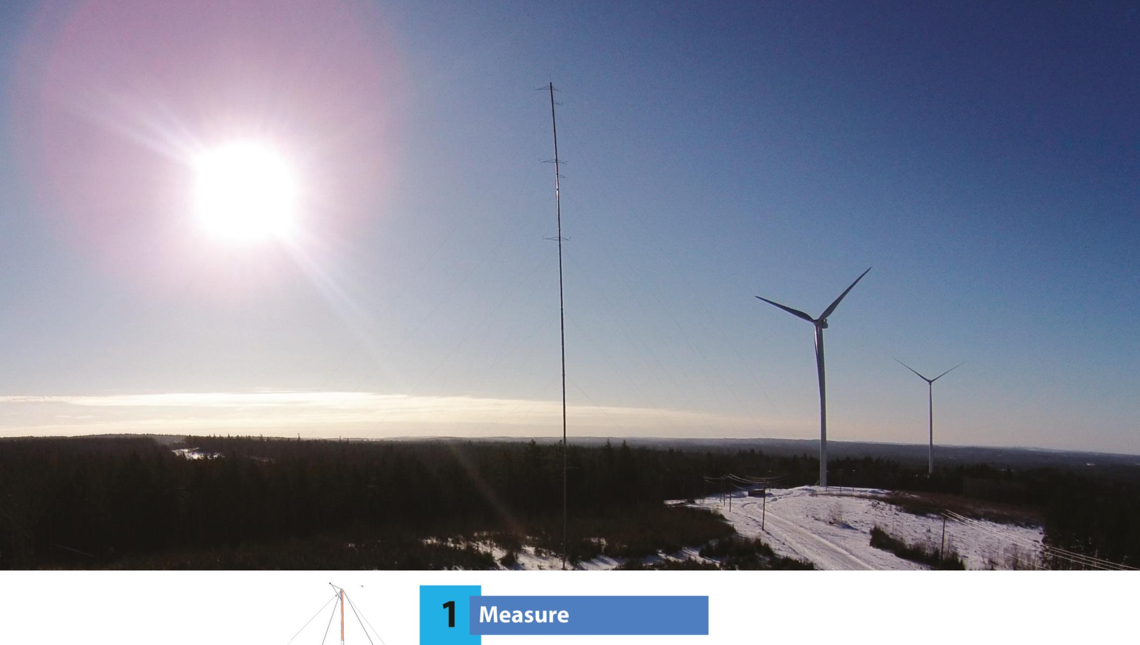
Meteorological test towers measure the wind speed, temperature, humidity, and barometric pressure over a full year.
